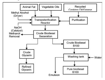
**Figure 1: Process Flow Sheet for Preparation of Biodiesel**
