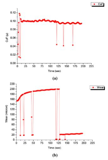
Figure 3 CoF Vs time b) Wear Vs time at 187 N load of sample 2
