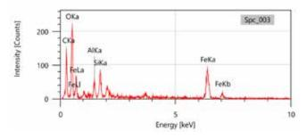
Figure 13 EDX graph of sample 3 after wear test
