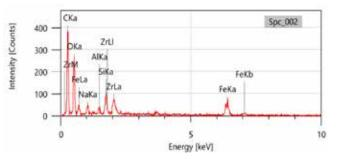
Figure 10 EDX graph of sample 2 after wear test
