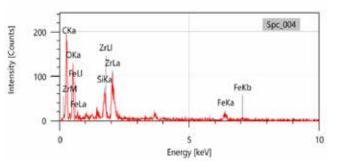
Figure 6 EDX graph of sample 1 before wear test
