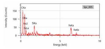
Figure 12 EDX graph of sample 3 before wear test
