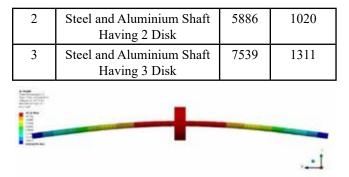
Figure 4. Modal analysis of Aluminum shaft Single disk system
