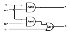
Figure 5: Logic diagram of carry generator stage
