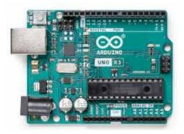
Figure 2 (a): Arduino UNO Board
