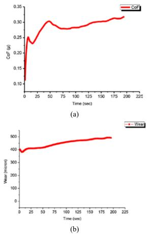
Figure 2 CoF Vs time b) Wear Vs time at 187 N load of sample 1
